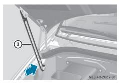
Swing the hood upwards until support strut
