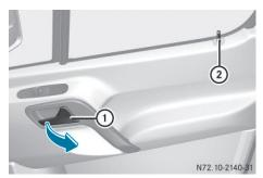
You can open the driver's or co-driver's door from the inside at any time, even if it is locked.
