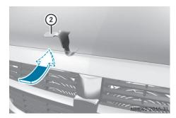
Reach into the gap and push grip ② on the hood catch upwards.
