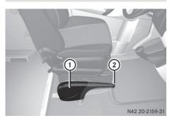
The brake lamps are not illuminated when you brake the vehicle using the parking brake. As a rule, you may only apply the parking brake when the vehicle is stationary.
