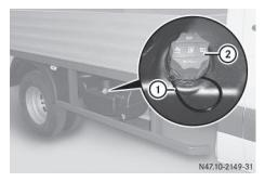
The DEF reservoir on the right-hand side of the vehicle (example: Cab Chassis)
