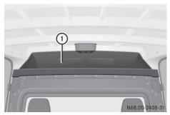
On vehicles with a partition, stowage space ① can only be loaded from the cargo compartment.
