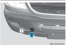
The fixture for the front towing eye is located in the bumper.
