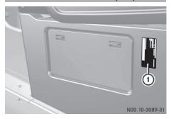
Vehicle identification plate for vehicles or chassis on the base of the driver's seat
