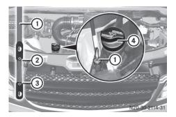
For vehicles with a red oil dipstick, only check the oil level when the engine is at normal operating temperature:
