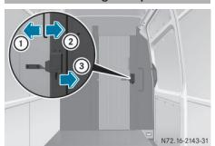
► To unlock: press the catch in the direction of arrow ③.
