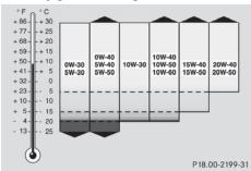
Using the chart below, select oil viscosity according to the lowest air temperature expected before the next oil change.
