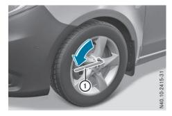
► Loosen the wheel bolts on the wheel to be changed in a counter-clockwise direction by about one turn using lug wrench ①. Do not remove the wheel bolts.
