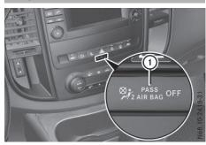
PASSENGER AIR BAG OFF indicator lamp (1) is part of the Occupant Classification System (OCS).
