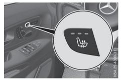
The three red indicator lamps in the  $\boxed{1}$  button show the activated heating level **1** to **3**.
