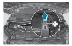
Push contact protection cover ① of the jumpstarting connection point backwards against the spring force as far as it will go. The jump-starting connection point is visible.
