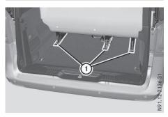
Example: seat rail system with quick-locking mechanism
