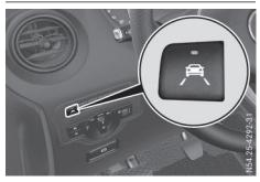
Press the Auton. If the indicator lamp in the button lights up and the display shows the A symbol in the status area, Lane Keeping Assist is switched on but not ready for use.
