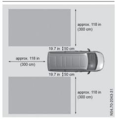
Blind Spot Assist monitors the area shown in the diagram up to 118 in (3 m) behind and directly next to your vehicle.
