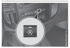
▶ Press the A ECO button. When the indicator lamp in the B ECO button lights up, the ECO start/stop function is activated.
