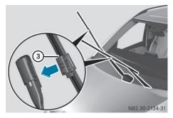
Insert new wiper blade (3) into the wiper arm in the direction of the arrow.
