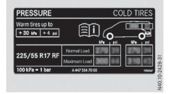
Tire pressure table inside the fuel filler flap (example: Cargo Van)
