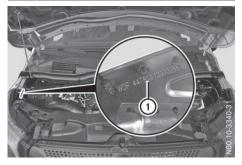
VIN in the engine compartment
