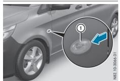
The additional turn signals are mounted on the side of the vehicle's front fender.
