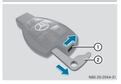
Slide release catch (1) in the direction of the arrow and, at the same time, remove mechanical key (2) from the key completely.
