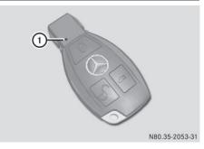
Press the g or g button. If battery check lamp () lights up briefly, the battery is sufficiently charged.
