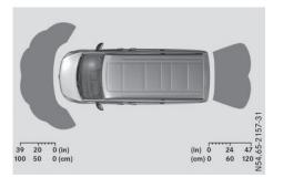
The sensors must be free of dirt, ice or slush. Otherwise, they cannot function correctly. Clean the sensors regularly, taking care not to scratch or damage them ( $\triangleright$  page 258).
