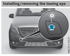
The fixture for the front towing eye is located in the bumper.
