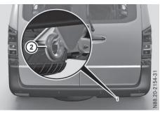
The rear towing eye is located under the bumper.
