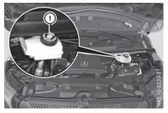
Check the brake fluid level regularly, e.g. weekly or when refueling.
