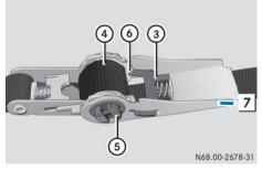
Tensioning lever in the release position
