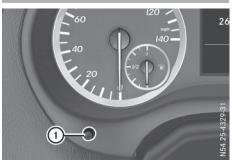
Brightness control knob (example: vehicle with steering wheel buttons)
