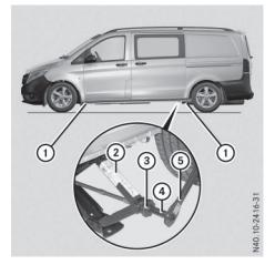
Jacking points (1) (rubber stoppers) are located just behind the front wheel arches and just in front of the rear wheel arches.
