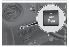
Press the press the button. If PARKTRONIC is deactivated, the indicator lamp in the switch lights up.
