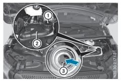
Example: cap and coolant expansion tank
