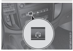
Press the <u>f</u> b program selector button repeatedly until the desired transmission program is selected.
