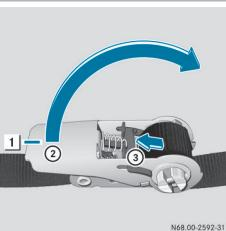
Tensioning lever fastened in detent position
