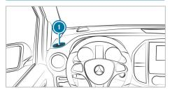
The ashtray with cap ① can be inserted into a cup holder on the cockpit or into a cup holder in the rear passenger compartment.
