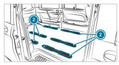
Seat anchorages with quick-locking mechanism (example: three seat anchorages per row of rear seats)
