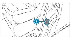
Vehicle identification plate ① is on the B-pillar on the driver's side.
