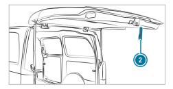
**To close:** pull the tailgate firmly downwards by loop (2) and close it from outside.
