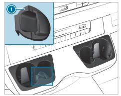
The cup holders for the driver and co-driver are in the center console.
