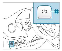
To prevent the electric parking brake from applying automatically, pull switch **()**.
