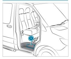
The hydraulic jack is located in side compartment (1) above the co-driver door step.
