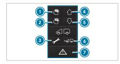
Electronic level control starts automatically if the ignition is switched on. Operation is only possible after the parking brake has been applied.
