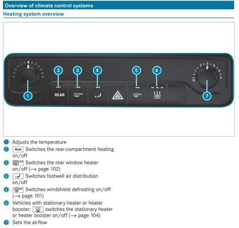
(i) The indicator lamps on the buttons signal that the function in question has been activated.
