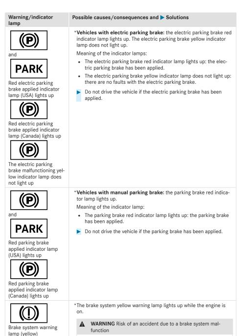
If the brake system is malfunctioning, braking characteristics may be impaired.
