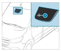
Active Lane Keeping Assist monitors the area in front of your vehicle by means of multifunction camera (). It serves to protect you against unintentionally leaving your lane. You may also be warned by a vibrating message from the steering wheel and by the status symbol flashing in the instrument display. In addition, you may be guided back into your lane by a lane-correcting brake application. A relevant message appears in the instrument display.
