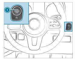
To switch on the power supply: press button ① once.
