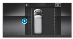
If a lane-correcting brake application from Active Lane Keeping Assist occurs, display **()** appears in the multifunction display.
