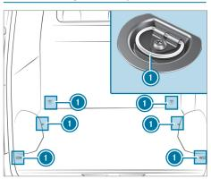
Cargo tie-down points (example: Cargo Van without loading rails)
