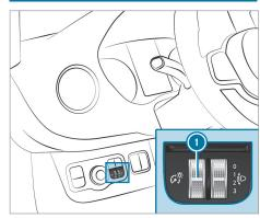
Turn brightness control () upwards or downwards.
