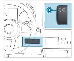
**To engage/disengage:** press the upper section of switch **()**.
