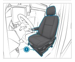
You can rotate the driver's and front passenger seats by  $50^{\circ}$  and  $180^{\circ}$ . The seats engage both in and opposite to the direction of travel as well as at  $50^{\circ}$  to the exit.
