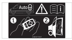
Warning notice, depending on the equipment on the driver's door, the partition wall, the sliding door or the Speed Delivery Door
