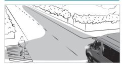
The cornering light improves the illumination of the road over a wide angle in the turning direction, e.g. enabling better visibility in tight bends.
