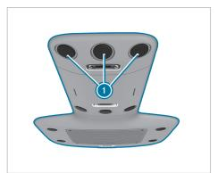
In vehicles with a rear air conditioning system, adjustable air vents have been integrated in the roof air duct.
