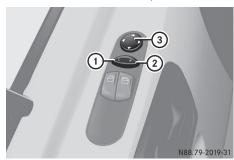
Button and switch for mirror adjustment
