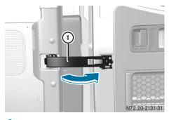
• Vehicles with 270° pivoting rear doors: If you prefer to keep door retainer • out of the loading area when loading the vehicle, you can swivel it 180° against the spring force and onto the door and engage it. The door retainer remains in this position and will not swivel back to its original
