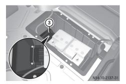
► Loosen the bolts holding retainer ③, which prevents the battery from moving around.
