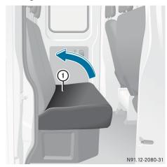
► To fold up the seat cushion: lift seat cushion ① out of the front anchorage and fold upwards in the direction of the arrow.
