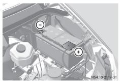
Additional battery in the engine compartment
