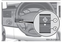
► To activate: press upper section ① of the ⊕ switch while the engine is running. The indicator lamp in the switch comes on. Vehicles without steering wheel buttons: The ADR indicator lamp in the instrument cluster lights up.
