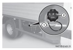
The DEF reservoir on the right-hand side of the vehicle (example: Cab Chassis)
