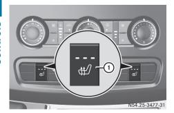
The three red indicator lamps in button (1) show the activated heating level 1 to 3.
