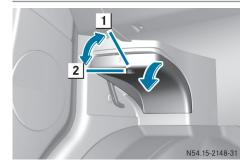
Fuse box in the footwell on the left-hand side of the vehicle.
