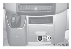
Socket on the lower section of the center console 1 12 V socket, 25 A
