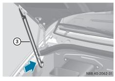
Swing the hood upwards until support strut3 engages and the hood is supported.
