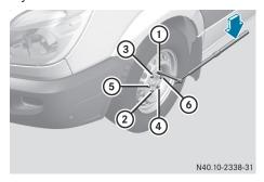
Tightening torque pattern
