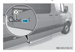
► Insert R-clips ② into the step as far as they will go through the holes on both sides of the housing.
