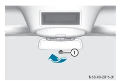
► Anti-glare mode: push anti-glare lever (1) in the direction of the arrow.
