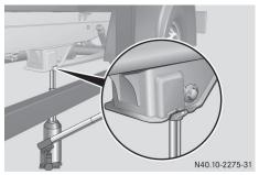
Jacking point (example: Cab Chassis)
