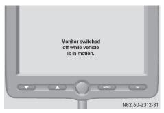
If the speed falls below 5 mph (8 km/h), the monitor switches on again.
