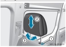
Head restraint (example: luxury head restraint on the co-driver's seat)
