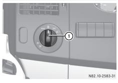
Light switch between driver's door and steering wheel
