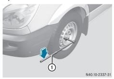
► Loosen the wheel nuts or wheel bolts on the wheel to be changed by about one turn using extended lug wrench (1). Do not unscrew the wheel bolts or wheel nuts completely.
