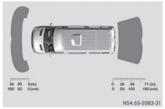
The sensors must be free of dirt, ice or slush. Otherwise, they cannot function correctly. Clean the sensors regularly, taking care not to scratch or damage them (> page 270).
