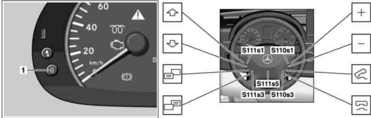
1. Switch on ignition. The total kilometers must be displayed in order to reach the "service scope x in xxx km" menu. Should the total kilometers not be shown in the display, press the system selection button in the lower control panel (S111s3) until the total kilometers are displayed.
