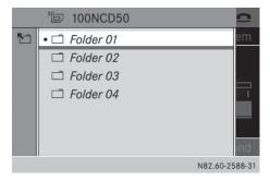
▶ Press the button. The display shows a list of folders on the first level. A • dot indicates the folder in which the track currently playing can be found.
