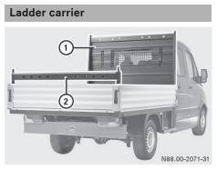
Example: ladder rack on Chassis Cab
