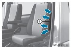
Side impact air bags ① deploy next to the outer bolster of the seat backrest.
