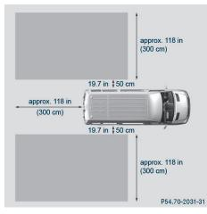
Blind Spot Assist monitors the area approximately 10 ft (3.0 m) behind your vehicle and approximately 1.6 ft (0.5 m) to 11.5 ft (3.5 m) each side of it. For this purpose, Blind Spot Assist uses radar sensors in the rear bumper and behind the protective strips of the B-pillars.
