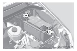
Additional battery in the engine compartment
