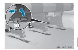
Locking mechanism lever on the feet of the bench seat
