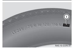
In addition to the load-bearing index, load rating () may be imprinted after the letters that identify speed rating on the sidewall of the tire ( $\triangleright$  page 261).
