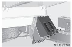
Wheel chock to the rear of the chassis on the left side of the vehicle (example)
