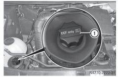
Example: DEF filler cap in the engine compartment
