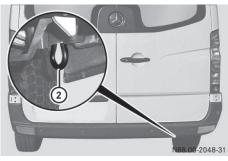
Rear towing eye under the bumper, attached to the chassis
