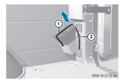
Wheel chock in the load/passenger compartment
