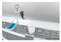
Reach into the gap and push lever (2) on the hood catch up.
