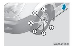
Tightening torque pattern
