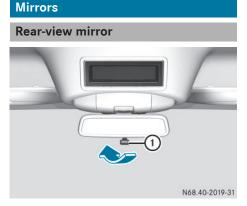
Anti-glare mode: push anti-glare lever 1 in the direction of the arrow.
