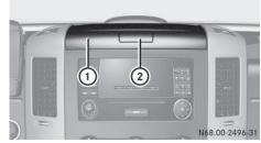
Stowage compartment on the dashboard above the center console (example with lid)
