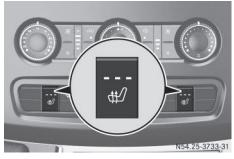
The three red indicator lamps in the # button show the activated heating level **1** to **3**.
