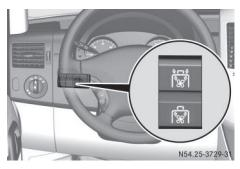
If your vehicle is equipped with a roof ventilator, you can ventilate and extract air from the cargo compartment.
