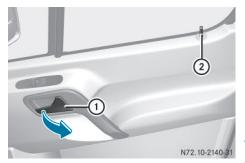
You can open the driver's or front-passenger door from the inside at any time, even if it is locked.
