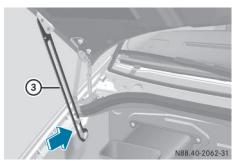
Swing the hood upwards until support strut
