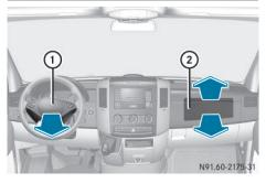
Driver's air bag ① deploys in front of the steering wheel. Front-passenger air bag ② deploys in front of and above the glove box and the center console.
