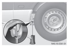
Jacking point, rear axle (example: vehicle type 2500)
