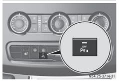
Press the prise button. If PARKTRONIC is deactivated, the indicator lamp in the switch lights up.
