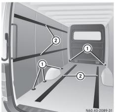
Cargo tie-down points (example: Cargo Van with loading rails)
