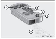
Remote control with an integrated folding key
