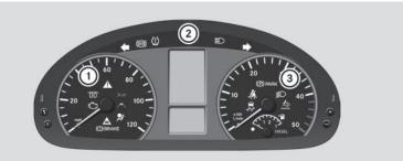
Instrument cluster in vehicles with steering-wheel buttons
