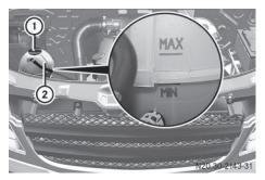
Example: cap and coolant expansion tank
