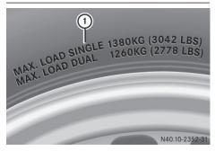
Maximum tire load ① is the maximum permissible weight for which the tire is approved. Do not overload the tires by exceeding the specified load limit. The maximum permissible load can be found on the vehicle's Tire and Loading Information placard on the B-pillar on the driver's side ( $\triangleright$  page 258).
