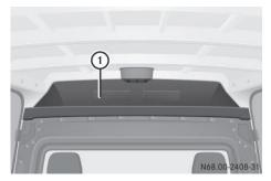
On vehicles with a partition, stowage space (1) can only be loaded from the cargo compartment.
