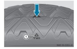
Bar marking ① for tread wear is integrated into the tire tread.
