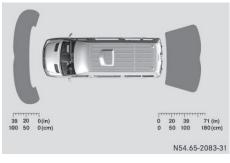
The sensors must be free of dirt, ice or slush. Otherwise, they cannot function correctly.
