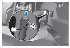
Battery main switch to the left of the center console
