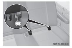
Install the LATCH-type (ISOFIX) child restraint system on both LATCH-type (ISOFIX) securing rings ①. ISOFIX is a standardized securing system for specially designed child restraint systems on the rear seats. LATCH-type (ISOFIX) securing rings ① for a LATCH-type (ISOFIX) child restraint system are installed between the seat cushion and the seat backrest:
