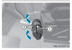
Fire extinguisher at the front of the base of the codriver's seat
