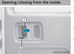
Release the lever on the inside of the right rear door
