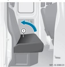
For vehicles with a crewcab, you can use the stowage compartment under the rear bench seat to safely store tools and other small items.
