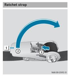
Tensioning lever fastened in detent position
