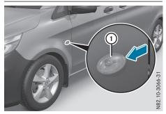
The additional turn signals are mounted on the side of the vehicle's front fender.
