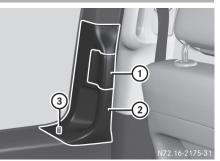
The sliding door is equipped with an active retainer, which engages the door at the end stop when opened.
