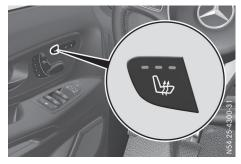
The three red indicator lamps in the bp button show the activated heating level **1** to **3**.
