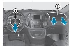
Driver's air bag ① deploys in front of the steering wheel. Front-passenger front air bag ② deploys in front of and above the glove box and the center console.
