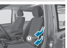
Side impact air bags (1) deploy next to the outer bolster of the seat backrest.
