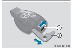
Slide release catch (1) in the direction of the arrow and, at the same time, remove mechanical key (2) from the SmartKey completely.
