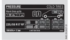
Tire pressure table inside the fuel filler flap (example: Passenger Van)
