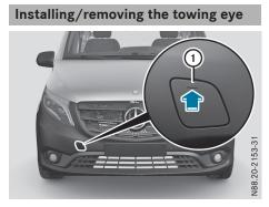
The fixture for the front towing eye is located in the bumper.
