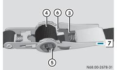
Tensioning lever in the release position
