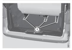
Example: seat rail system with quick-locking mechanism
