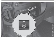
▶ Press the <a>Press the <a>ECO</a> ECO button. When the indicator lamp in the <a>ECO</a> button lights up, the ECO start/stop function is activated.
