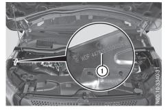
VIN in the engine compartment
