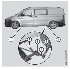
Jacking points () (rubber stoppers) are located just behind the front wheel arches and just in front of the rear wheel arches.
