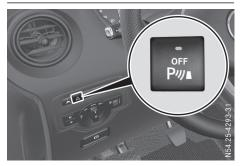
Press the press the press the press the press the press the press button. If PARKTRONIC is deactivated, the indicator lamp in the switch lights up.
