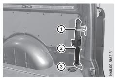
Holder for the jack in the cargo compartment on the right-hand side of the vehicle
