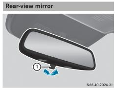
Anti-glare mode: push anti-glare lever (1) forwards or back.
