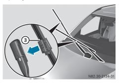
Insert new wiper blade (3) into the wiper arm in the direction of the arrow.
