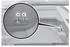
Stowage compartment equipped with smartphone connections
