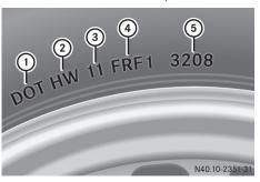
The TIN is a unique identification number. The TIN enables the tire manufacturers or retreaders to inform purchasers of recalls and other safety-relevant matters. It makes it possible for the purchaser to easily identify the affected tires. The TIN is made up of manufacturer identification code ②, tire size ③, tire type code ④ and manufacturing date ⑤.
