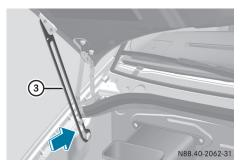
► Swing the hood up until support strut ③ engages and the hood is supported.
