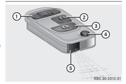
Remote control with an integrated folding key
