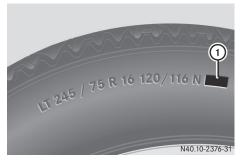
In addition to the load-bearing index, load rating ① may be imprinted after the letters that identify speed rating on the sidewall of the tire (> page 258).
