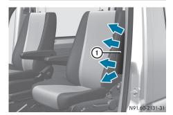
Side impact air bags (1) deploy next to the outer bolster of the seat backrest.
