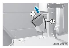
Wheel chock in the load/passenger compartment
