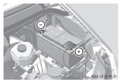
Additional battery in the engine compartment
