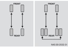
Diagram showing tire rotation for single and dual
