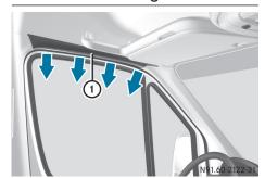
Window curtain air bags (1) are integrated into the side of the roof frame above the front doors. When deployed, the window curtain air bag enhances the level of protection for the head. However, it does not protect the chest or arms. In the event of a side impact, the window curtain air bag is deployed on the side on which the impact occurs.
