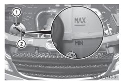
Example: cap and coolant expansion tank
