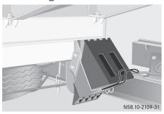
Wheel chock to the rear of the chassis on the left side of the vehicle (example)
