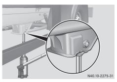
Jacking point, rear axle (example: Cab Chassis)
