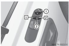
Adjustment buttons and switches for setting the mirrors
