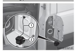
The fuel filler flap is beside the front left-hand door when viewed in the direction of travel. It is only possible to open the fuel filler flap when the front door is open.
