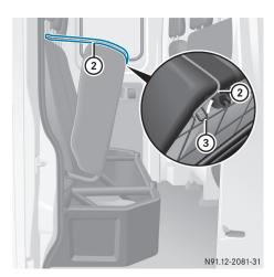
Retainer loops ② are secured to the outer head restraints.
