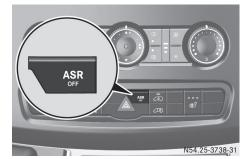
When ESP® is intervening and the warning lamp in the instrument cluster is flashing, leave ASR on. In this case, only depress the accelerator pedal as far as required when pulling away.
