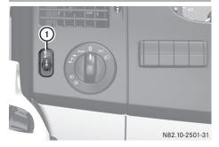
The headlamp range control is used to adapt the downward angle of the headlamp beams in accordance with the load on your vehicle. The cone of light from the headlamps changes if seats are occupied or if the cargo compartment is being loaded or unloaded. This can impair visibility and cause glare to oncoming traffic.
