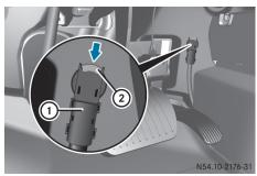
Battery main switch to the left of the center console
