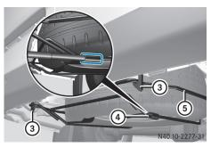
Spare wheel carrier under the vehicle
