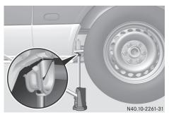
Jacking point, rear axle (example: vehicle type 2500)
