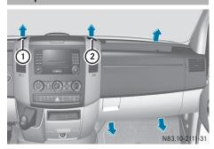
Air vents (example: right-hand side of the vehicle)
