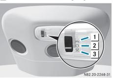
Interior light with switch (example: Passenger Van with rear-compartment air conditioning)
