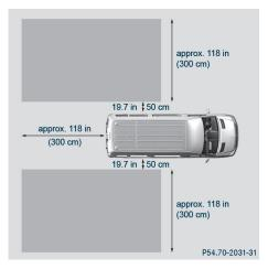
Blind Spot Assist monitors the area approximately 10 ft (3.0 m) behind your vehicle and approximately 1.6 ft (0.5 m) to 11.5 ft (3.5 m) each side of it. The monitoring range behind the vehicle may also be larger depending on the situation.
