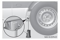
Jacking point, rear axle (example: vehicle type 3500)
