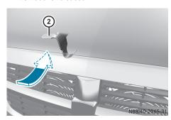
▶ Reach into the gap and push lever ② on the hood catch up.
