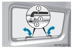
The emergency exit window is intended for use in an emergency only and must not be opened unless the vehicle is stationary. The emergency exit window is the first window behind the driver's seat on the driver's side. It is marked by the "Emergency Exit" label.
