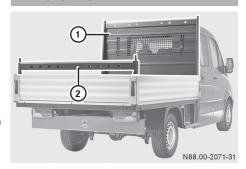
Example: ladder rack on Chassis Cab
