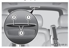
Rear area warning display in center of headliner in rear compartment.
