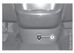
When the key is turned to position 1 in the ignition lock, the sockets can be used for accesso-
