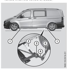
Jacking points (1) (rubber stoppers) are located just behind the front wheel arches and just in front of the rear wheel arches.
