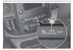
PASSENGER AIR BAG OFF indicator lamp (1) shows you whether the front-passenger front air bag is deactivated.
