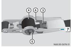
Tensioning lever in the release position
