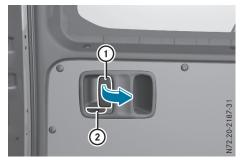
Release the lever on the inside of the right rear door A white section on latch ② indicates that the rear door is unlocked.
