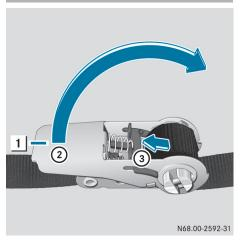
Tensioning lever fastened in detent position
