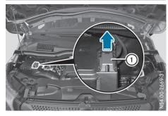
Push contact protection cover ① of the jumpstarting connection point backwards against the spring force as far as it will go.
