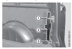
Holder for the jack in the cargo compartment on the right-hand side of the vehicle
