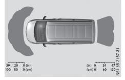
The sensors must be free of dirt, ice or slush. Otherwise, they cannot function correctly. Clean the sensors regularly, taking care not to scratch or damage them (> page 266).
