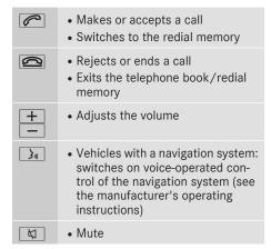
1 The audio devices, telephone and voiceoperated control using the steering wheel buttons in the right control panel only function with a Mercedes-Benz audio or navigation system. If you are using an audio or navigation system from another manufacturer, the described functions may be restricted or not available at all.
