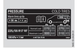
Tire pressure table inside the fuel filler flap (example: Cargo Van)
