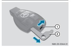
▶ Slide release catch (1) in the direction of the arrow and, at the same time, remove mechanical key (2) from the SmartKey completely.
