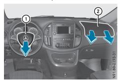
Driver's air bag ① deploys in front of the steering wheel. Front-passenger front air bag ② deploys in front of and above the glove box and the center console.
