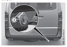
The rear towing eye is located under the bumper. If you tow or tow-start a vehicle, attach the towing device to rear towing eye (2).
