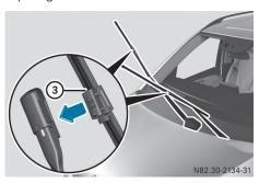
► Insert new wiper blade ③ into the wiper arm in the direction of the arrow.
