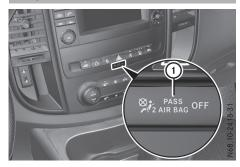
PASSENGER AIR BAG OFF indicator lamp ① is part of the Occupant Classification System (OCS).
