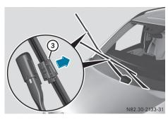
► Remove wiper blade ③ from wiper arm by pulling it in the direction of the arrow.
