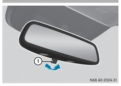
► Anti-glare mode: push anti-glare lever ① forwards or back.
