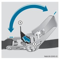
Threading and tensioning
