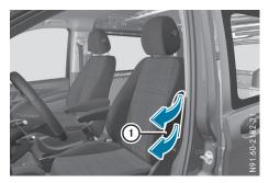
Side impact air bags ① deploy next to the outer bolster of the seat backrest.
