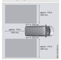
Blind Spot Assist monitors the area shown in the diagram up to 118 in (3 m) behind and directly next to your vehicle.
