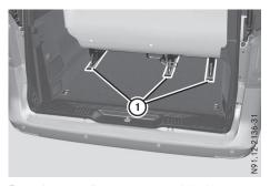
Example: seat rail system with quick-locking mechanism
