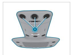
In vehicles with rear-compartment air conditioning, adjustable air vents have been integrated in the roof air duct.
