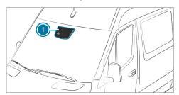
Traffic Sign Assist detects traffic signs with multifunction camera 1. It assists you by displaying detected speed limits and overtaking restrictions in the instrument cluster.
