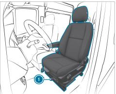
You can rotate the driver's and co-driver's seat 50 ° and 180 °. The seats engage both in and opposite to the direction of travel as well as at 50 ° to the exit.
