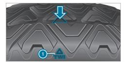
Markings show in which places the bar indicators (arrow) are integrated into the tire tread. They are visible as soon as the tread depth is approximately ½ 16 in (1.6 mm).
