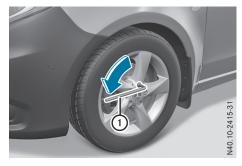
► Using lug wrench (1), loosen the wheel bolts on the wheel to be changed counter-clockwise by about one full turn. Do not remove the wheel bolts.
