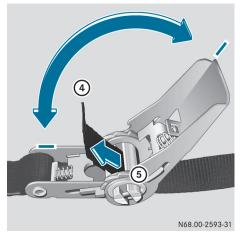
Threading and tensioning
