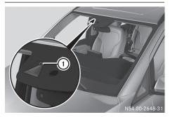
Lane Keeping Assist monitors the area in front of your vehicle by means of camera ① which is mounted at the top of the windshield. Lane Keeping Assist detects lane markings on the road and can warn you before you leave your lane unintentionally.
