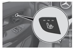
The three red indicator lamps in the b button show the activated heating level **1** to **3**.
