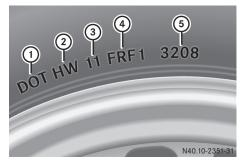
The TIN is a unique identification number. The TIN enables the tire manufacturers or retreaders to inform purchasers of recalls and other safety-relevant matters. It makes it possible for the purchaser to easily identify the affected tires. The TIN is made up of manufacturer identification code (2), tire size (3), tire type code (4) and manufacturing date (5).
