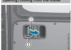
Release the lever on the inside of the right rear door
