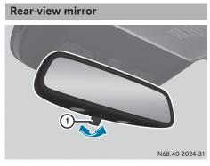
Anti-glare mode: push anti-glare lever (1) forwards or back.
