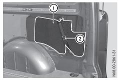
Tool holder in the cargo compartment on the righthand side of the vehicle
