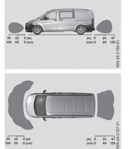
The sensors must be free of dirt, ice or slush. Otherwise, they cannot function correctly. Clean the sensors regularly, taking care not to scratch or damage them ( $\triangleright$  page 266).
