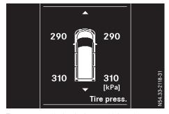
Tire pressure display (only on vehicles with steering wheel buttons)
