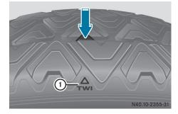
Marker (1) shows the location where the bar indicator (arrow) for tread wear is integrated into the tire tread.
