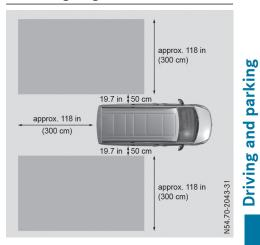
Blind Spot Assist monitors the area shown in the diagram up to 118 in (3 m) behind and directly next to your vehicle.
