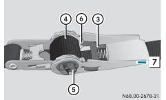
Tensioning lever in the release position
