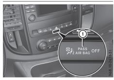
PASSENGER AIR BAG OFF indicator lamp (1) shows you whether the front-passenger front air bag is deactivated.
