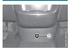
When the key is turned to position 1 in the ignition lock, the sockets can be used for accessories with a maximum power consumption of 180 W (15 A).
