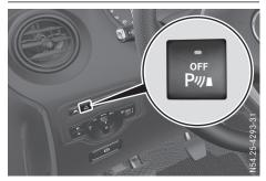
Press the press the button. If PARKTRONIC is deactivated, the indicator lamp in the switch lights up.
