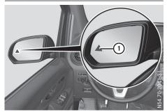
Blind Spot Assist is not active at speeds below approximately 20 mph (30 km/h). Vehicles in the monitoring range are then not indicated.
