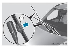
Remove wiper blade ③ from wiper arm by pulling it in the direction of the arrow.
