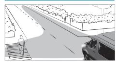
The cornering light improves the illumination of the roadway over a wide angle in the turning direction, e.g. enabling better visibility in tight bends. The function is active under the following conditions:
