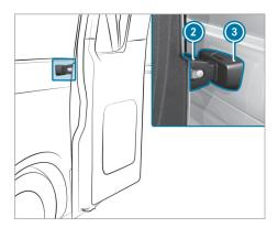
With the rear-end door opened 270°, push it against magnetic door retainer (3) on the side wall.
