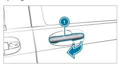
The sliding door is equipped with an active retainer, which engages when the door is opened as far as it will go.
