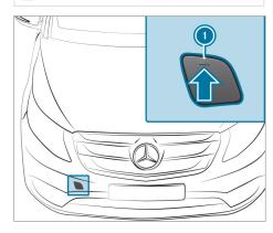
Fixture for the front towing eye in the bumper
