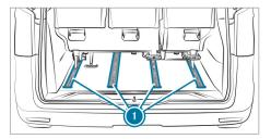
Example: seat rail system with quick-locking mechanism
