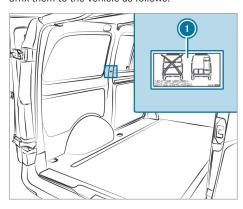
Clean the surface before sticker is affixed. The stickers must be affixed to a flat, metallic surface free from grease and dust. Affix stickers on every side of the vehicle in close proximity to the loading rails in a clearly visible location.
