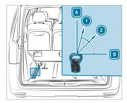
Example: lashing angle for optimal load security
