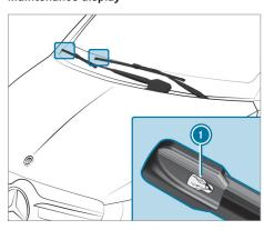
Remove protective film from the maintenance displays on the tips of the newly installed wiper blades.
