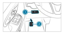
If, in exceptional cases, the service brake fails, you can use the parking brake to perform emergency braking.
