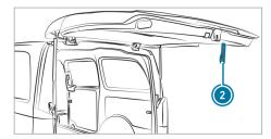
**To close:** pull the tailgate firmly downwards by loop ② and close it from outside.
