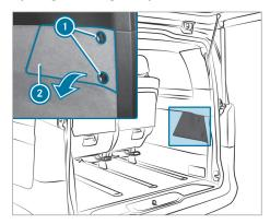
Storage compartment in the rear compartment on the right-hand side of the vehicle
