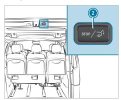
Press button ② in the tailgate and step out of the swinging range of the tailgate.
