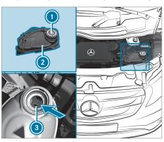
Example: cap and coolant expansion reservoir
