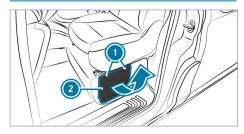
Storage compartment in the seat base of the left front seat
