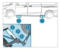
Jacking points (1) (rubber stoppers) are located behind the front wheel arches and in front of the rear wheel arches.
