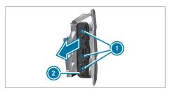
Unscrew three screws 1 and remove bulb mount 2 from the tail lamp.
