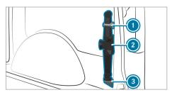
Holder for jack in the cargo compartment on the right-hand side of the vehicle (for example, Cargo Van)
