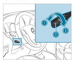
Turn controller 3 in direction 2 to increase the specified minimum distance and in direction 1 to reduce the specified minimum distance.
