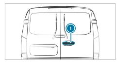
You can stop the rear-end doors at an angle of approximately 90°, and also at 180° or 270°. Make sure that the opened rear-end door is stopped correctly in the catch.
