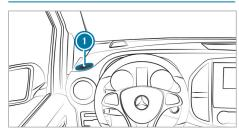
► The ashtray with cap (1) can be inserted into a cup holder on the cockpit or into a cup holder in the rear passenger compartment.
