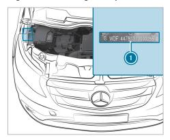
VIN (1) is engraved into the longitudinal member in the engine compartment next to the fuse box.
