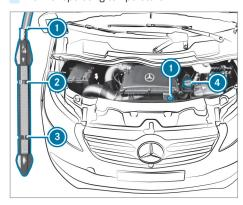
Oil dipstick and engine oil filler opening (example: gasoline engine)
