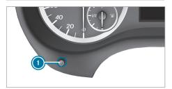
Brightness control (example: vehicle with steering-wheel buttons)
