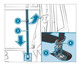
Floor anchorage (example: secured tie-down eye)
