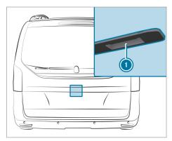
Press button in the handle and step out of the swinging range of the tailgate.
