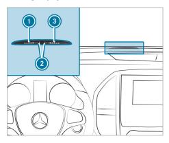
Front area warning display on the center of the cockpit
