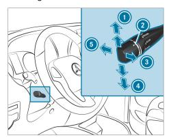
To activate with the current speed: briefly press the cruise control lever briefly up ① or down ② and take your foot off the accelerator pedal.
