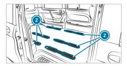
Seat anchorages with quick-locking mechanism (example: three seat anchorages per row of rear seats)
