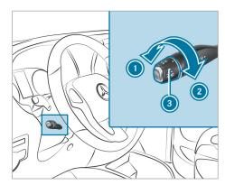
➤ Turn controller ③ in direction ② to increase the specified minimum distance and in direction ④ to reduce the specified minimum distance.
