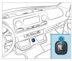
Opens and closes the sliding door on the right side of the vehicle
