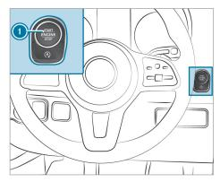
To switch on the power supply: press button (1) once.
