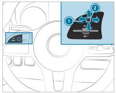
The on-board computer is operated via left-hand Touch Control ② and back button on the left ①.
