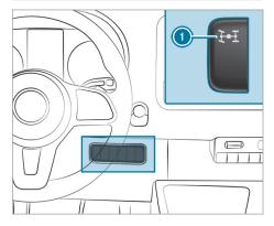
To engage/disengage: press the upper section of switch (1).
