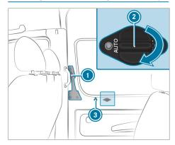
If there has been a malfunction or if the battery has been disconnected, you can use disconnect switch ② to disconnect the sliding door from the electric motor. Then you can open or close the door manually.
