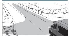
The cornering light improves the illumination of the roadway over a wide angle in the turning
