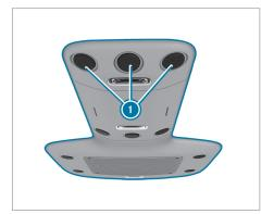
In vehicles with a rear compartment air conditioning system, adjustable air vents have been integrated in the roof air duct.
