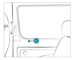
When the sliding door is locked, it can only be opened from the inside by manually unlocking locking pin (a).
