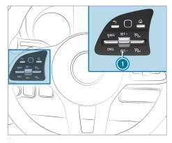
Brake or accelerate the vehicle to the desired speed on the downhill gradient. Release the brake or accelerator pedal. The current speed is stored.
