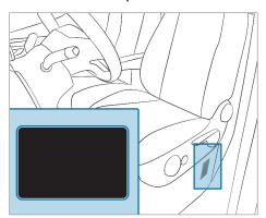
Depending on the vehicle model, the vehicle identification plate is located on the seat base of the driver's seat or on the B-pillar.
