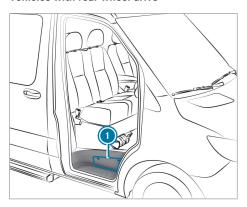
The tire-change tool kit is located in stowage compartment
