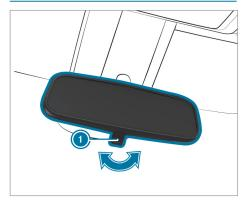
Fold anti-glare lever in the direction of the arrow.
