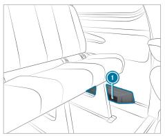
Depending on the vehicle equipment, there will be an air duct or a heater with additional air vents in the rear compartment footwell on the left-hand side 1. No objects may be placed there. Occupants must maintain a sufficient distance due to the warm air flow and air intake.
