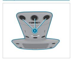
In vehicles with a rear air conditioning system, adjustable air vents are integrated in the roof air duct.
