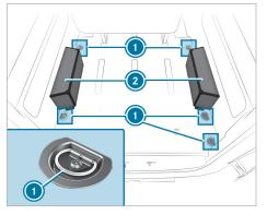
Place the objects on wheel arch ② and lash them using tie-down eyes ① (→ page 211). (i) A wheel arch may be subjected to a load of 330 lb (150 kg).
