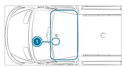
Position of the key holder when the detection range of the antenna is reduced
