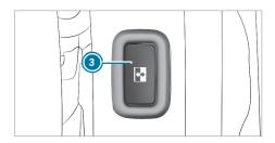
On vehicles with a partition, the button (§) is located on the partition next to the door entrance at the height of the inside door handle.
