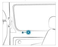
When the sliding door is locked, it can be opened only from the inside by manually unlocking locking pin (a).
