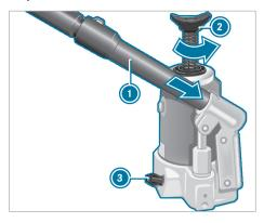
To prepare the hydraulic jack: insert the third rod of pump lever for the jack into the lug wrench extension.
