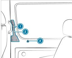
Pull safety pin (a) upwards manually or use the central locking button to unlock the sliding door (→ page 50).
