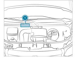
Engraved VIN (1) is located underneath the hood.
