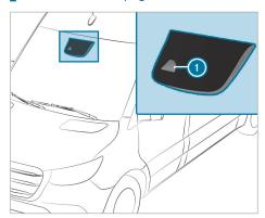
Lane Keeping Assist monitors the area in front of your vehicle with multifunction camera ①. It serves to protect you against unintentionally leaving your lane. You may also be warned by a noticeable vibration in the steering wheel or by a warning tone and by the status symbol flashing on the instrument cluster.
