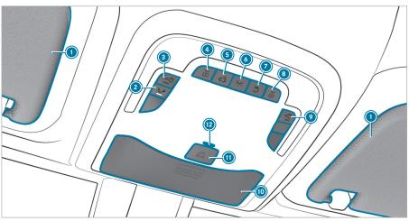
Overhead control panel for vehicles with bus equipment 6 Switches the front interior Sun visors lighting on/off call button Switches the rear interior 88 lighting on/off Activates/deactivates the → 88 bus function reading light on/off reading light on/off Switches reading lights in the 88 passenger compartment on/off Switches automatic light 88 control on/off Eyeglasses compartment
