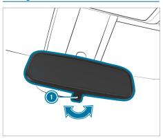
Fold anti-glare lever in the direction of the arrow.
