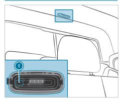
Switches rear passenger compartment/ cargo compartment lamp on or off
