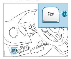
The electric parking brake is also automatically applied if Active Distance Assist DISTRONIC has brought the vehicle to a standstill.
