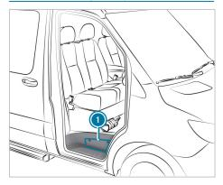
The hydraulic jack is located in side compartment  $\bar{\ }$
