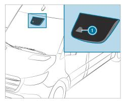
Active Lane Keeping Assist monitors the area in front of your vehicle by means of multifunction camera . It serves to protect you against unintentionally leaving your lane. You may also be warned by a noticeable vibration in the steering wheel or by a warning tone and by the status symbol flashing in the instrument cluster. In addition, you may be guided back into your lane by a lane-
