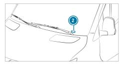
The VIN is also attached as a label at the lower end of the windshield 2.
