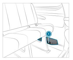
Depending on the vehicle equipment, there will be an air duct or a heater with additional air vents in the rear footwell on the left-hand side ①. No objects may be placed there. Occupants must maintain a sufficient distance due to the warm air flow and air intake.
