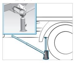
Jack support point, rear axle (example: chassis up to 3.5 t)
