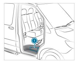
The tire-change tool kit is located in stowage compartment ① above the step of the front passenger door and in the stowage compartment in the footwell on the front passenger side.
