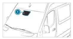
Traffic Sign Assist detects traffic signs with multifunction camera ①. It assists you by displaying detected speed limits and overtaking restrictions on the instrument cluster.
