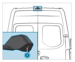
If you have activated the function in the multimedia system, the image from rear view camera (1) will appear in the multimedia system when reverse gear is selected. Dynamic guide lines show the path the vehicle will take for the current steering movement. This will help you to orient yourself and to avoid obstacles when backing up.
