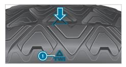
Markings • show in which places the bar indicators (arrow) are integrated into the tire tread. They are visible as soon as the tread depth is approximately  $\frac{1}{16}$  in (1.6 mm).
