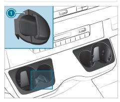
The cup holders for the driver and front passenger are in the center console.
