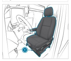
You can rotate the driver's and front passenger seats by 50° and 180°. The seats engage both in and opposite to the direction of travel as well as at 50° towards the exit.
