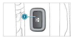
In vehicles with a partition, button () is located on the partition next to the door entrance at the height of the inside door handle.
