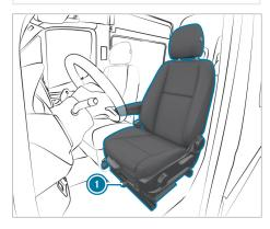
You can rotate the driver's and front passenger seats by  $50^{\circ}$  and  $180^{\circ}$ . The seats engage both in and opposite to the direction of travel as well as at  $50^{\circ}$  towards the exit.
