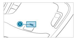
When the ATA system is armed, an indicator lamp (1) flashes in the overhead control panel.
