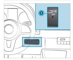
The reverse warning device is a system designed to assist you in ensuring the safety of other road users. The reverse warning device cannot guarantee that no persons or objects are situated behind the vehicle.
