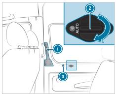
If there has been a malfunction or if the battery has been disconnected, you can use disconnect switch ② to disconnect the sliding door from the electric motor. Then you can open or close the sliding door manually.
