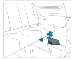
Depending on the vehicle equipment, there will be an air duct or a heater with additional air vents in the rear footwell on the left-hand side
