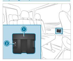
Place the mobile phone in storage compartment and connect it to USB port to charge.
