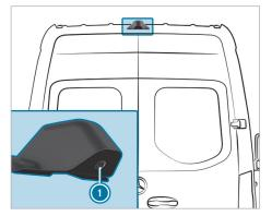
If you have activated the function in the multimedia system, the image from rear view camera 1 will appear in the multimedia system when reverse gear is selected. Dynamic guide lines show the path the vehicle will take for the current steering movement. This will help you to orient yourself and to avoid obstacles when backing up.
