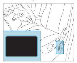
Depending on the vehicle model, the vehicle identification plate is located on the seat box of the driver's seat or on the B-pillar.
