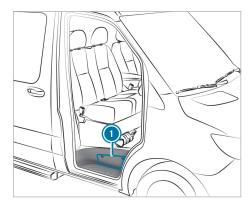
The tire-change tool kit is located in stowage compartment 1 above the step of the front passenger door and in the stowage compartment in the footwell on the front passenger side.
