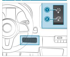
If your vehicle is equipped with a roof ventilator, you can admit fresh air to the cargo compartment, and extract air from it as well.
