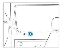
When the sliding door is locked, it can only be opened from the inside by manually unlocking locking pin (4).
