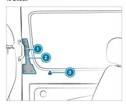
Pull safety pin (3) upwards manually or use the central locking button to unlock the sliding door ( $\rightarrow$  page 52).
