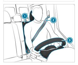
Ensure the following when adjusting steering wheel ③, seat belt ② or driver's seat ①:
