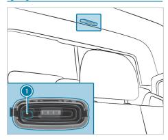
Switches rear passenger compartment/ cargo compartment lamp on or off
