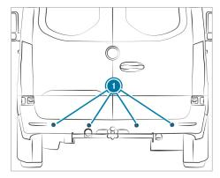
Certain driving and driving safety systems use sensors (1) to monitor the area in front of, behind or next to the vehicle (depending on the vehicle's equipment).
