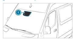
Traffic Sign Assist detects traffic signs with multifunction camera (1). It assists you by displaying detected speed limits and overtaking restrictions on the instrument cluster.
