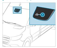
Lane Keeping Assist monitors the area in front of your vehicle with multifunction camera 1. It serves to protect you against unintentionally leaving your lane. You may also be warned by a noticeable vibration in the steering wheel or by a warning tone and by the status symbol flashing on the instrument cluster.
