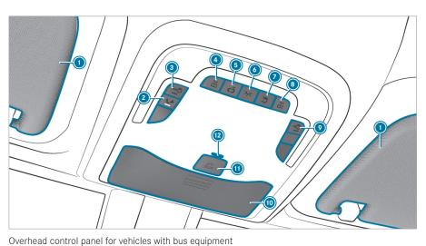
Sun visors Switches the rear interior lighting on/off call button 3 Switches the right-hand reading light on/off ③ Activates/deactivates the → bus function Activates/deactivates reading lighting in the passenger com-partment reading light on/off Eyeglasses compartment Switches automatic light control on/off
