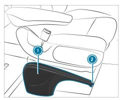
If, in exceptional cases, the service brake fails, you can use the parking brake to perform emergency braking.
