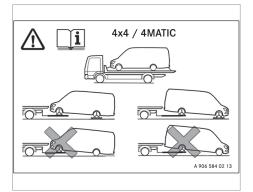
Vehicles with all-wheel drive: warning notice on the B-pillar on the driver's side
