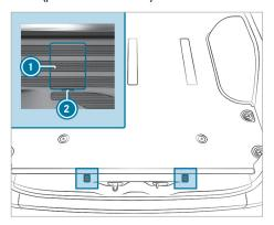
Bolt covers for the retaining hooks (example: panel
