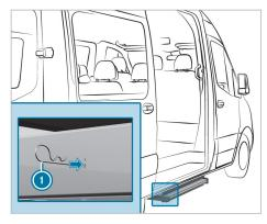
On both sides, insert spring cotters (1) through the housing's holes and into the step as far as they will go.
