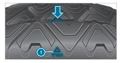
Markings n show in which places the bar indicators (arrow) are integrated into the tire tread. They are visible as soon as the tread depth is approximately  $V_{16}$  in (1.6 mm).
