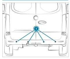
Certain driving and driving safety systems use sensors () to monitor the area in front of, behind or next to the vehicle (depending on the vehicle's equipment).
