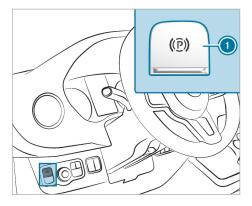
The electric parking brake is also automatically applied if Active Distance Assist DISTRONIC has brought the vehicle to a standstill and the driver is not sitting in the driver's seat.
