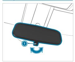
Fold anti-glare lever ① in the direction of the arrow.
