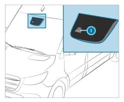
Active Lane Keeping Assist monitors the area in front of your vehicle by means of multifunction camera (). It serves to prevent you from unintentionally leaving your lane. You may also be warned by a noticeable vibration in the steering wheel or by a warning tone and by the status symbol flashing on the instrument cluster. In addition, you may be guided back into your lane by a lane-correcting brake application. A corresponding message will appear on the instrument cluster.
