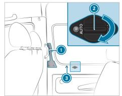
If there has been a malfunction or if the battery has been disconnected, you can use disconnect switch ② to disconnect the sliding door from the electric motor. Then you can open or close the sliding door manually.
