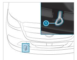
Press the top of the cover and remove the cover.
