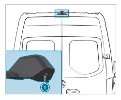
If you have activated the function in the multimedia system, the image from rear view camera () will appear in the multimedia system when reverse gear is selected. Dynamic guide lines show the path the vehicle will take for the current steering
