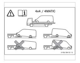
Vehicles with all-wheel drive: warning notice on the B-pillar on the driver's side
