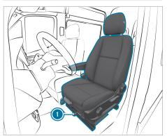
You can rotate the driver's and front passenger seats by  $50^{\circ}$  and  $180^{\circ}$ . The seats engage both in and opposite to the direction of travel as well as at  $50^{\circ}$  towards the exit.
