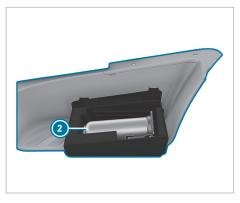
Remove jack (2) and the pump lever rod.
