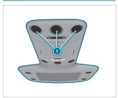
In vehicles with a rear air conditioning system, adjustable air vents have been integrated in the roof air duct.
