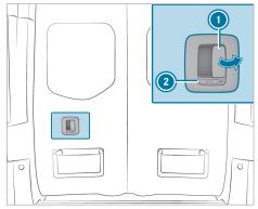
The **g** symbol indicates that the rear-end door is unlocked.
