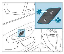
Central locking buttons (vehicles with manually adjustable front seats)
