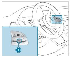
Turn volume control (). The volume of the current radio or media source is set. The volume of other audio sources can be adjusted separately.
