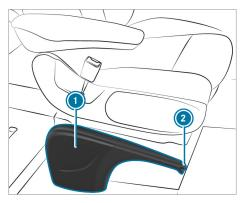
If, in exceptional cases, the service brake fails, you can use the parking brake to perform emergency braking.
