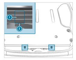
Bolt covers for the retaining hooks (example: panel van)
