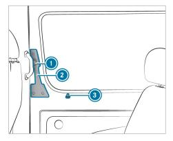
Pull safety pin (③) upwards manually or use the central locking button to unlock the sliding door (→ page 51).
