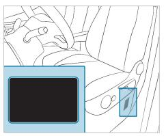
Depending on the vehicle model, the vehicle identification plate is located on the seat box of the driver's seat or on the B-pillar. (i) The data is vehicle-specific and may differ from that shown. Always observe the specifications on your vehicle identification plate.
