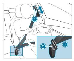
Always engage the seat belt tongue () of the seat belt into the seat belt buckle (2) of the corresponding seat.
