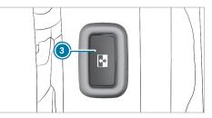
In vehicles with a partition, button (3) is located on the partition next to the door entrance at the height of the inside door handle.
