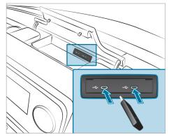
The multimedia connection unit is located at the top center of the stowage compartment and has two type C USB ports.
