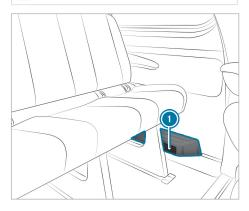
Depending on the vehicle equipment, there will be an air duct or a heater with additional air vents in the rear footwell on the left-hand side (). Do not place any objects here. Vehicle occupants must maintain a sufficient distance due to the warm air flow and air intake.
