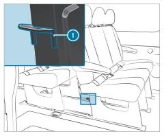
Top Tether anchorages () are located on the back of the rear bench seat on the bench seat legs.
