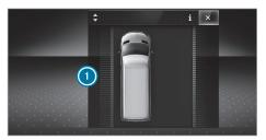
If a lane-correcting brake application from Active Lane Keeping Assist occurs, indicator () will appear on the instrument cluster display.
