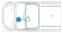
Position of the key holder when the detection range of the antenna is reduced
