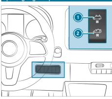
If your vehicle is equipped with a roof ventilator, you can admit fresh air to the cargo compartment, and extract air from it as well.
