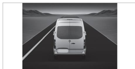
If a front wheel moves onto a detected lane marking, this is highlighted in red on the instrument cluster display in the **Assistance** menu.
