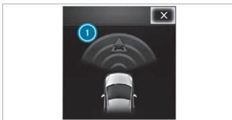
If an autonomous brake application or situation-dependent brake force boosting is implemented, the pop-up 1 appears on the instrument cluster display. It then automatically disappears after a short time.
