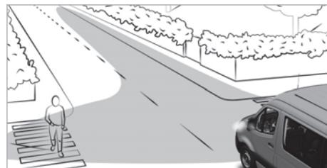
The cornering light improves the illumination of the road over a wide angle in the turning direction, e.g. enabling better visibility in tight bends.
