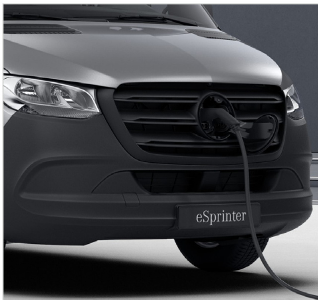
Position of the vehicle socket in the eSprinter model series 907
