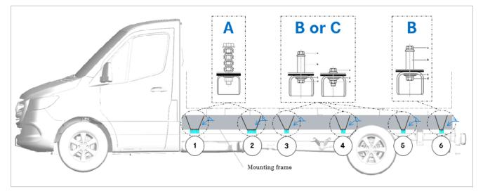
Sprinter cab chassis with 144" wheelbase - recommended attachment to the chassis frame/longitudinal members
