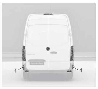
Rear of vehicle - speckled areas: Areas where wrapping is not permissible (example cargo van model designation, schematic diagram)
