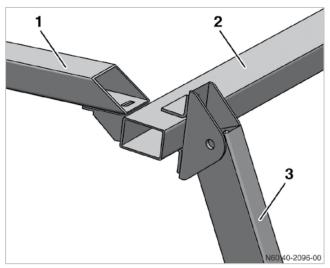
Additional connection of the longitudinal tubes
