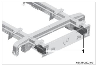
Longitudinal member on BM 907 Cab Chassis with code Q11  $\,$
