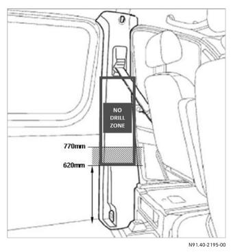
Location of seat belt retractor between 620-770 mm/ 24.25-30.5 in above floor
