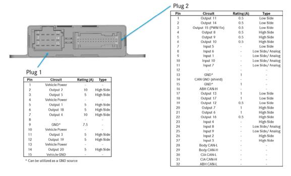
Pin Assignment of the PSM (MPM)
