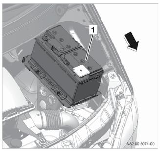
E2M: Auxiliary battery in engine compartment
