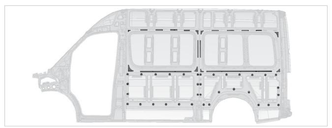
Cargo van model designation, inside of right side wall: Permissible areas for the attachment of load compartment trim parts (dark markings, schematic diagram)
