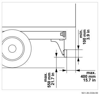
Side view of the rear underrun protection location
