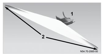
Positions of sensors of Blind Spot Assist (ISO layout)
