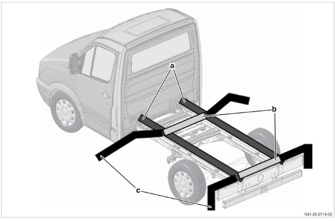
Attachment of assembly frame to body consoles
