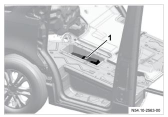
Schematic installation position of the main battery
