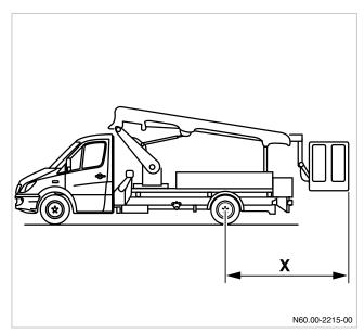
Maximum overhang lengths (using a lifting work platform as illustration)
