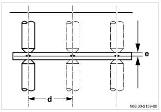
Ratio of sheet thickness to distance between spot welds
