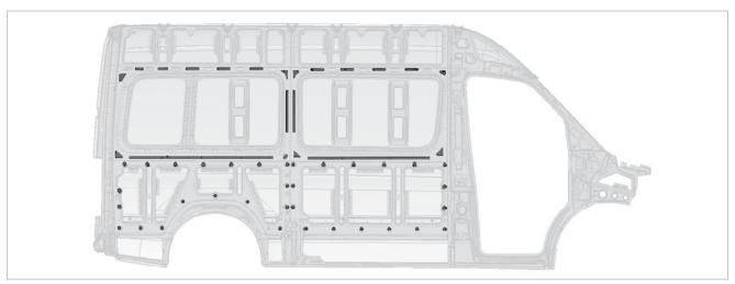
Cargo van model designation, inside of left side wall: Permissible areas for the attachment of load compartment trim parts (dark markings, schematic diagram)
