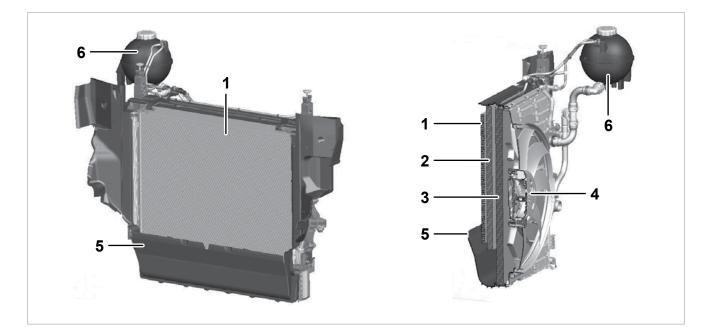
Cooling module for engine OM654
