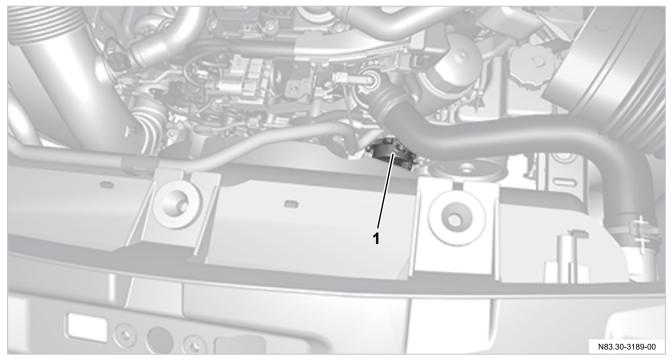
Position of belt tensioner in engine compartment
