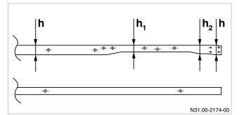
Dimensions of the lower flange of the longitudinal frame member
