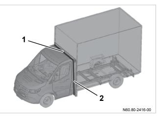
Attachment of body to B-pillar and roof (example of free-standing body, schematic diagram)
