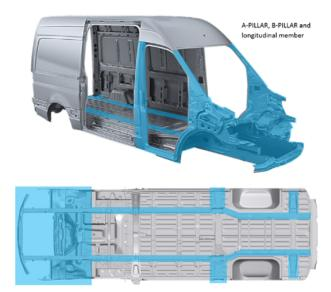
Safety and crash relevant areas (marked in blue) The diagram below shows where drilling into the longitudinal member is not allowed. Drilling must not take place:
