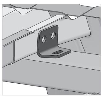
Connecting the shelf longitudinal tube to the roof bow bracket
