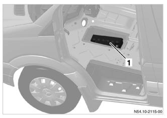
Installation position of the main battery
