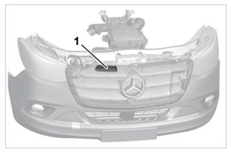
Engine air intake opening for OM654
