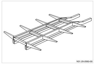
Example of a floor assembly design
