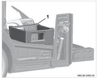
Schematic diagram of reinforced seat base
