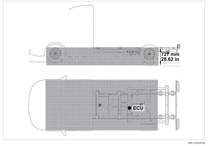
Restricted areas for tire pressure monitoring system (applies for both versions of the system used in the Sprinter)
