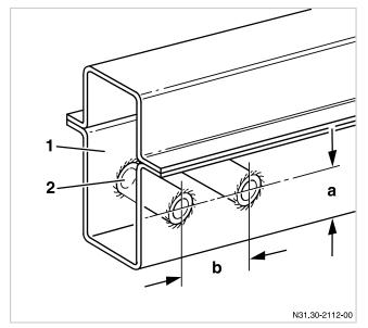
Drilling work on the longitudinal frame members (at the rear end only)
