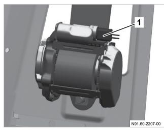
Retractor with pyrotechnical seat belt tensioner
