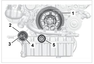
Belt tensioner on engine OM654 in as-delivered state (with code N63)
