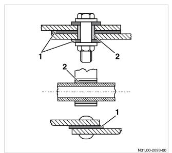
Preventing contact corrosion
