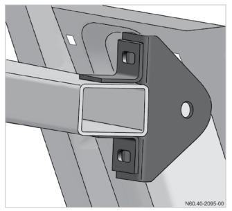
Connecting the longitudinal tube to the support
