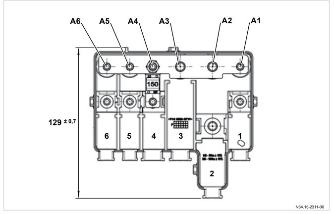
Assignment of fuse box (top view)
