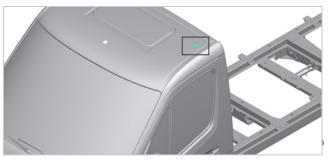
Position of antenna for the cab chassis
