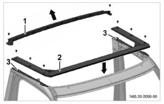
Mounting of auxiliary roof frame
