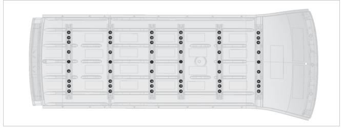
Cargol van model designation, inside of roof: Permissible areas for the attachment of load compartment trim parts at the cross bows (dark markings, schematic diagram)
