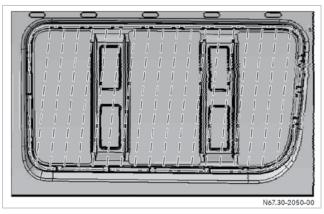
Example for cargo van/passenger van side wall body in white structure and glass area
