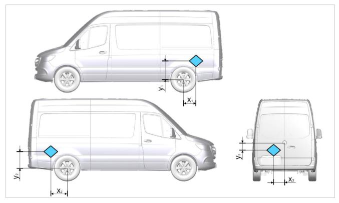
Positioning of placard holders (left, right, and rear position
