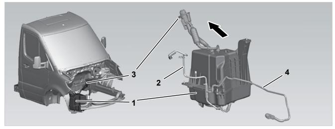
SCR system for engine OM654
