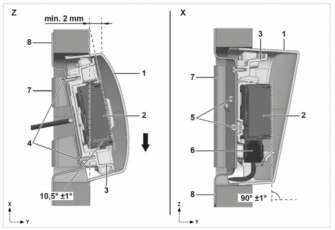
Schematic illustration of assembly on vehicle: Horizontal section (left, Z plane), Vertical section (right, X plane)
