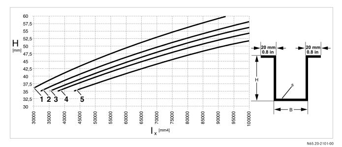
Required moments of inertia for roof bows with 20 mm/0.8 in flange with the roof skin
