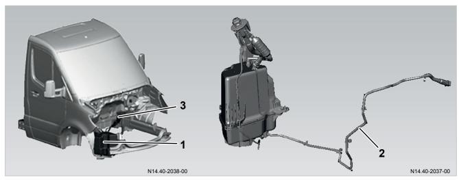
SCR system for engines OM651 / OM642
