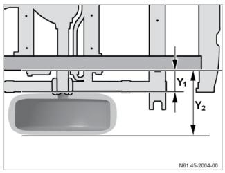
The diagram below shows the reference edges for the dimensions  $Y_1$  and  $Y_2$  on vehicles with tapering frame section (twin tires).
