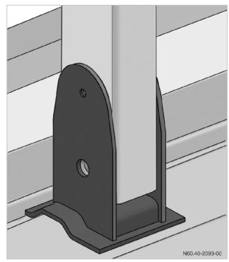
Bolting the mounting consoles to the floor
