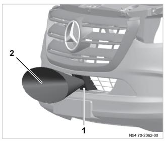
Position of Active Brake Assist sensor
