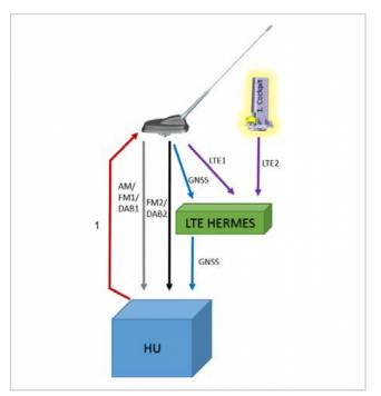
Connection diagram: Vehicles with ex factory antenna
