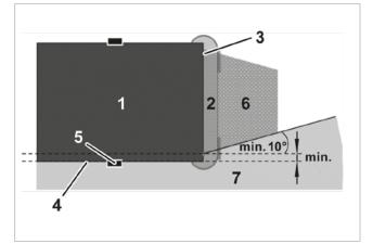
Positioning of the radar sensor system, possible installation positions at the rear
