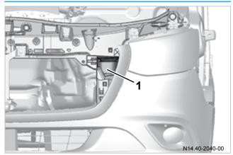
Engine air intake opening for OM651 / OM642
