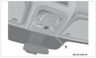
Position of SOS button in overhead control panel
