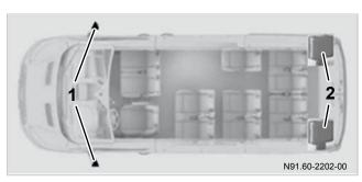
Sensor positions of Blind Spot Assist (schematic based on example of passenger van)
