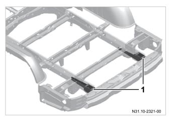
Longitudinal member on BM 907 Crew, Passenger and Cargo Van model with code Q11  $\,$
