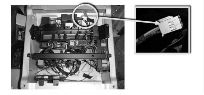
Trailer brake control preparation driver seat box
