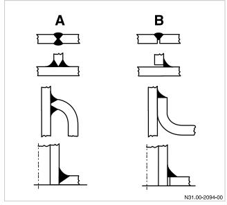
Examples of types of weld joints
