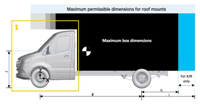
The following diagrams and tables show the general and the maximum side surface areas of Sprinter cab chassis vans. The point of origin for the dimensions as well as for the 3D data (available for eXpertUpfitters on www.UpfitterPortal.com) is located in the middle of the front axle.
