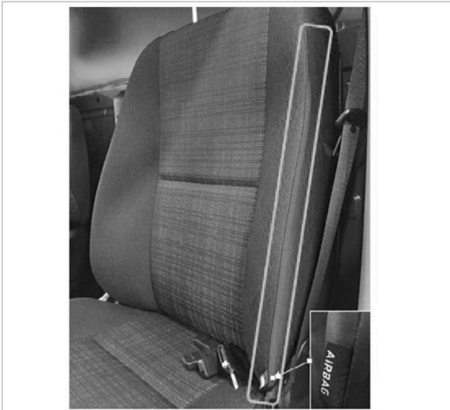
Front Seat with integrated Thorax-Pelvis-Airbag
