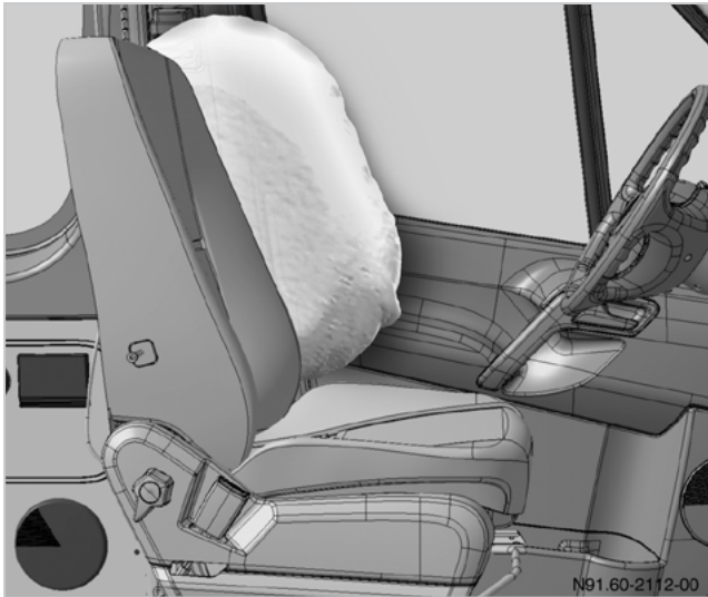
Schematic diagram of deployment area of thorax/pelvis side airbag on left side of vehicle
